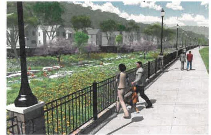
Waterway Access Path (Looking South toward Westwood) This image depicts the character of the proposed urban waterway through the Urban Ravine. The waterway contains a heavily-vegetated riparian edge, trees, and limestone rock. The height of the retaining wall from Westwood is visible. A pedestrian railing and lighting along the maintenance path and overlooks are included for safety (and as required by code).
