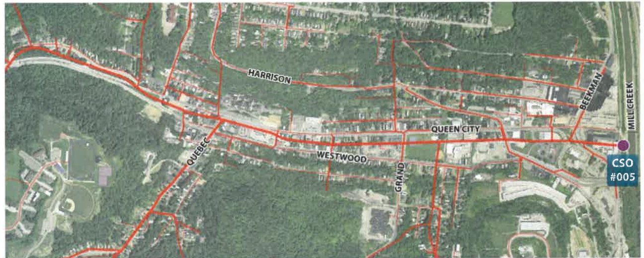
Existing Conditions in South Fairmount: Combined Sewer Conditions
