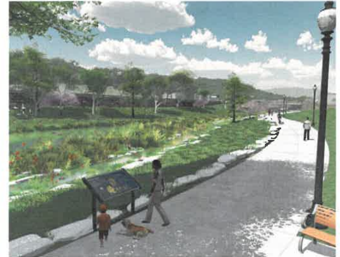
Eastern Gateway Zone (Looking South toward Westwood) This image depicts the character of the proposed urban waterway at the water quality feature. The multi-purpose path provides safe, well-lit access. During low volume rain events, runoff flows north of the water quality feature to Mill Creek. During high volume rain events, water flows both north of and into the water quality feature. This feature provides valuable terrestrial and aquatic habitat.
