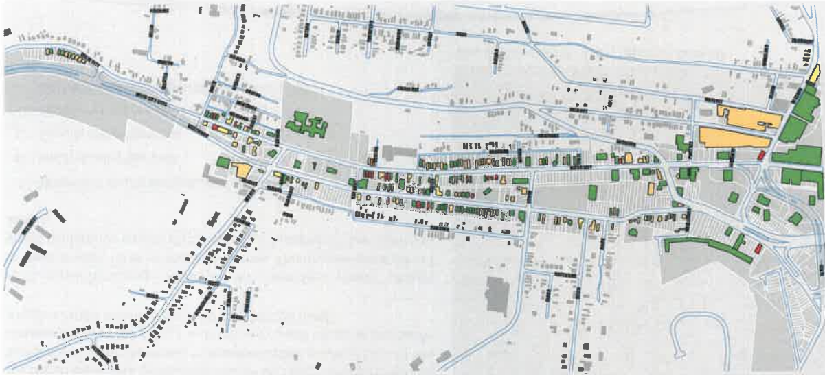
The Urban Audit assessed the exterior physical conditions of 244 buildings in the South Fairmount project area. The rating system included the following four categories: "Sound Condition," "Requires Minor Repair," "Requires Major Repair," and "In Critical Condition." The Survey form also required building information on frontage orientation to the street, height, and construction material.
